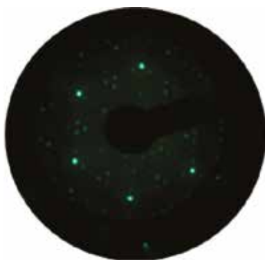
Image 5 Diffraction pattern of the pure silicon surface
