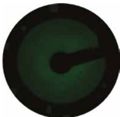
Image 4 Absence of a diffraction pattern on the silicon dioxide layer
