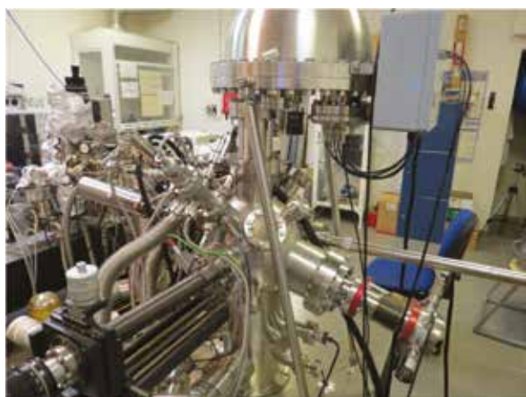
Image 1 The XPS machine used in the investigation
