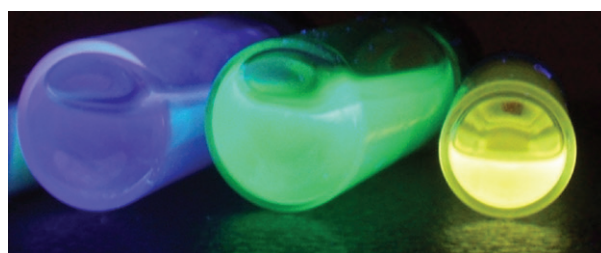
Figure 3b As an illustration the DCS emission is shown here in hexane, acetonitrile and HFIP with 360 nm wavelength excitation
