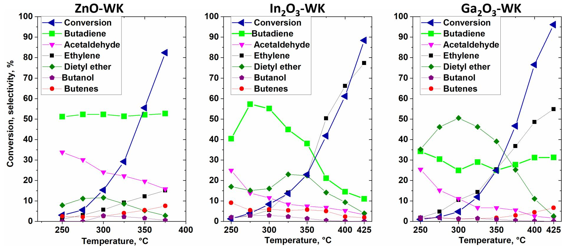
1 g catalyst, 0.5 g ethanol/(g<sub>cat</sub>\*h), 30 ml/perc (4.4 ml/min ethanol + 25.6 ml/min He)
