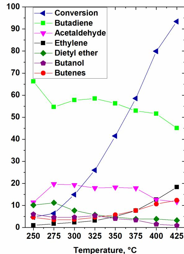
1 g catalyst, 0.5 g ethanol/(g<sub>cat</sub>\*h), 30 ml/perc (4.4 ml/min ethanol + 25.6 ml/min He)
